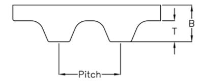
Height B mm= 2.2Height T mm= 1.2Length= 500Number of teeth= 100Pitch= 5Type= PU 25 T5 500Width= 25
